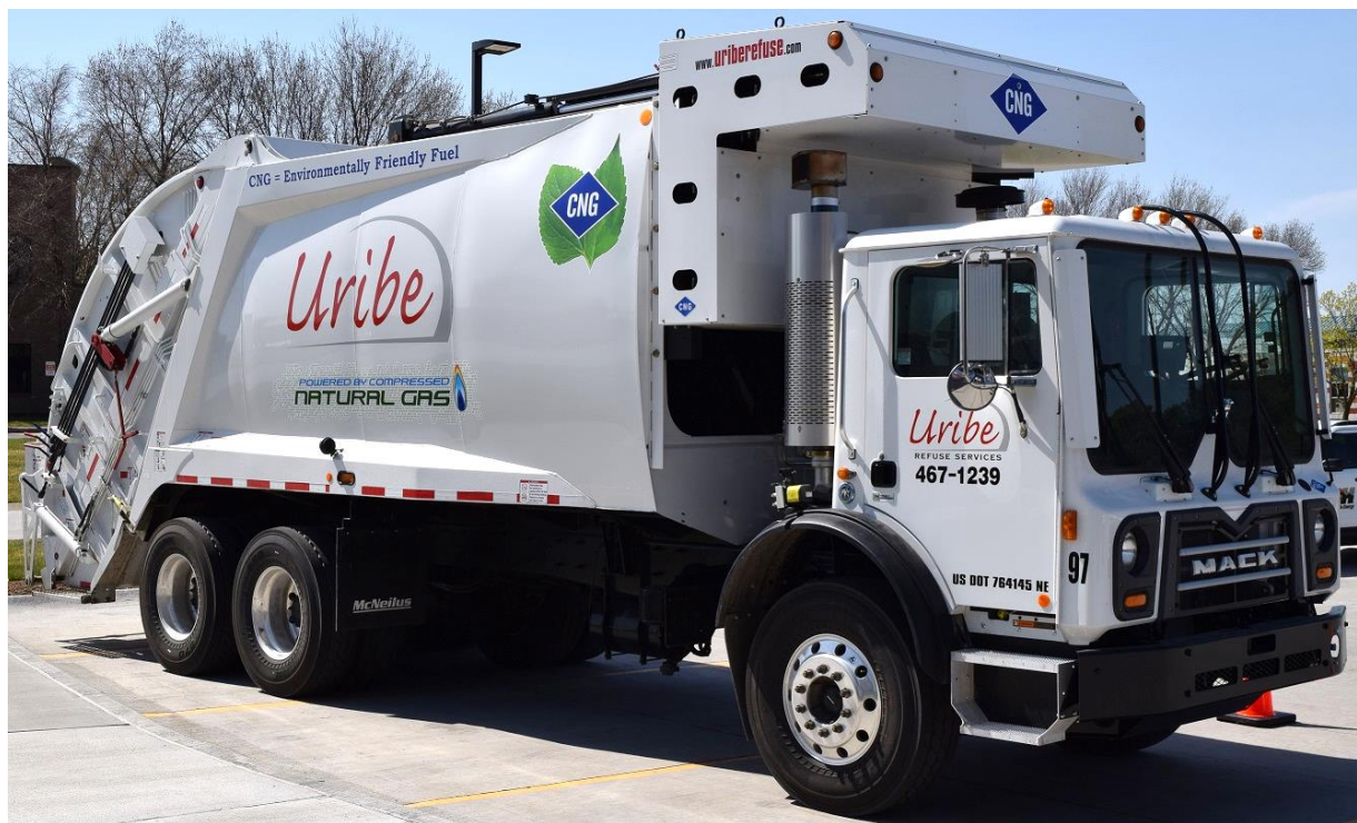
Cleaner replacement refuse truck powered by compressed natural gas (CNG) delivered to Uribe Refuse Services in Lincoln in May 2022, partially funded by the 2020 Nebraska Clean Diesel Rebate Program. NDEE photo.
