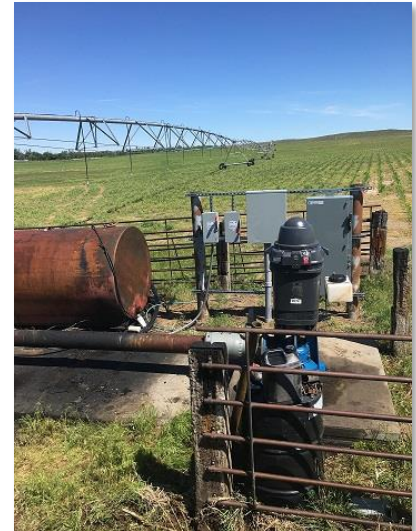
Diesel irrigation engine removal. Torch cutting hole in engine block. New electric motor in place.
