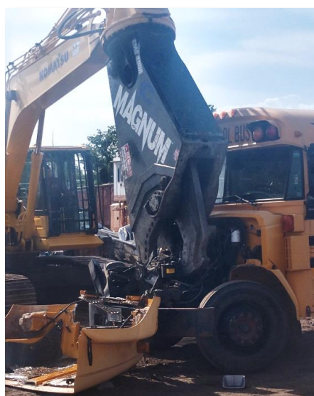
Above, chassis and engine of old school bus being scrapped.
