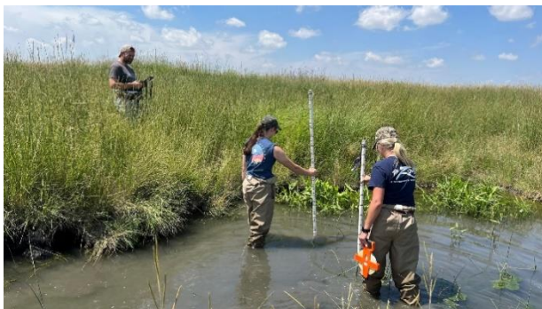
Conducting stream transect measurements
