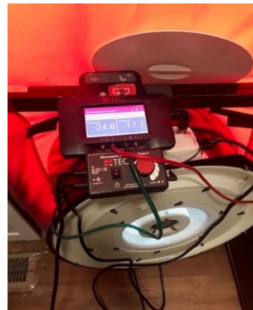
New Energy Efficient Housing, Gibbon (Buffalo County Assessor, 2021), Blower Door Testing (November 2021).
