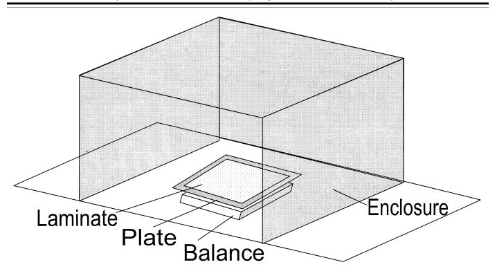
Figure 17.1. Typical Balance Enclosure
