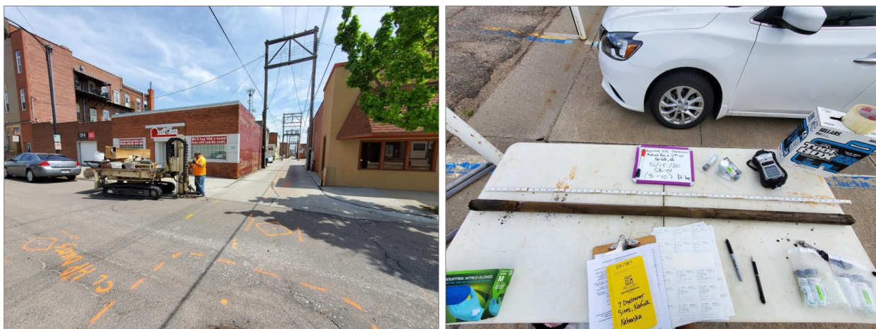
The photo on the left shows the collection of a soil boring using direct-push technology near a former dry-cleaning facility. The photo on the right shows the soil core from one boring location (photos courtesy of Tetra Tech).
