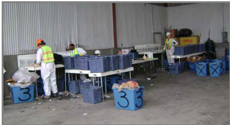
PHOTOGRAPH 2.2 SORTING AREA CONFIGURATION AT A TRANSFER STATION
