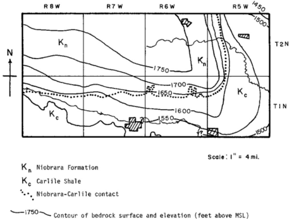
Figure 6: Contour map of upper bedrock surface, study area (Redrawn from Miller et al., 1964)
